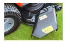
Side Discharge your Grass Cobra side discharge tractors feature a 42" cutting deck which allows the grass to be evenly discharged to the side of the machine as it mows. This is especially useful for cutting tall, thicker grass or for
