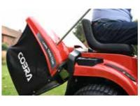
The high-performance collection system is largely achieved by a combination of the optimised grass chute, an efficient grass bag design and increased airflow created by the high quality twin bladed
