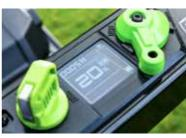
**LCD Operator Display Screen** An LCD display screen is integrated into the control panel. This screen gives the user essential information, including travel speed, the real-time power status of your batteries and a summary of your working time via an hour meter.
